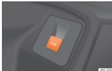
Fig. 82 On the driver's door: button to open and close the rear lid.
