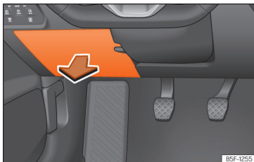
Fig. 220 On the dashboard on the driver side: lid of the fuse box.
