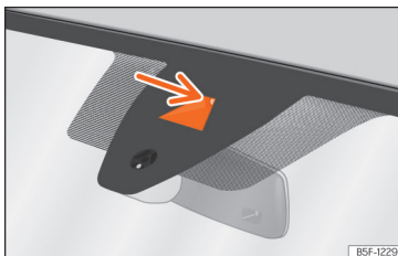
Fig. 129 On the windscreen: field of vision of the Lane Assist system camera.
