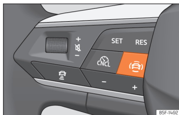
Fig. 126 Left side of the multifunction steering wheel: button for driver assistance systems (depending on the version).
