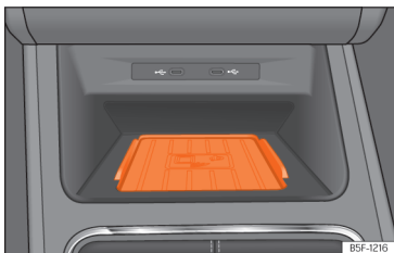
Fig. 176 On the centre console: pad for the mobile phone connection.
