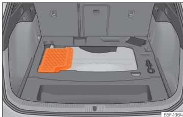
Fig. 235 Hybrid vehicles (PHEV): location of the battery in the luggage compartment
