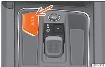
Fig. 69 Centre console (with automatic transmission): vehicle key housing.
