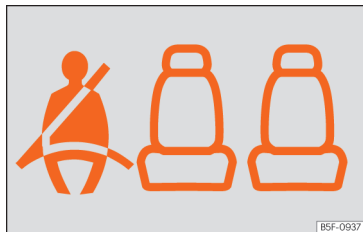
Fig. 17 Instrument cluster: indication of the status of the rear seat seat belts.
