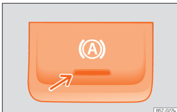
Fig. 132 In the lower part of the centre console: Auto Hold function button.
