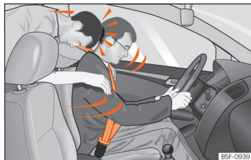
Fig. 20 Any rear seat occupants not wearing a seat belt may be thrown forward violently, hitting the driver who is wearing the seat belt.
