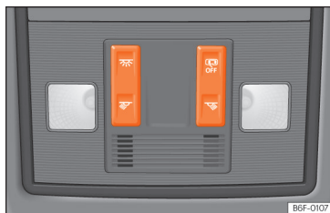
Fig. 71 Detail of headliner: front interior lighting.
