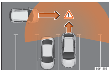
Fig. 130 Diagram of the parking assistant: detected area around the vehicle that is driving off.
