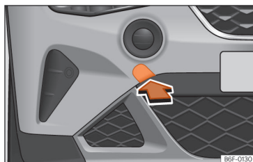
Fig. 164 Front bumper on right: remove the lid.
