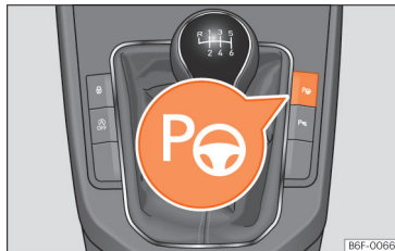
Fig. 123 In the centre console: button to switch on the Park Assist system.
