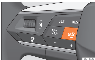
Fig. 91 Left side of the multifunction steering wheel: button for driver assistance systems (depending on the version).
