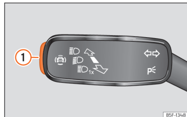
Fig. 90 On the turn light and main beam lever: key for driver assistance systems [depending on the version].
