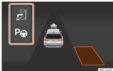
Fig. 124 On the instrument cluster display: display of the assisted parking system with decreased visibility.
