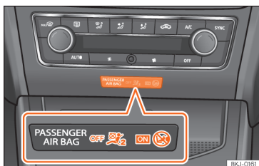
Fig. 28 Centre of the instrument panel: control lamp for deactivated front passenger airbag in centre console.
