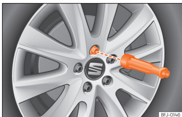
Fig. 257 Changing the wheel: unscrew wheel bolts with the socket at the end of the wheel brace.
