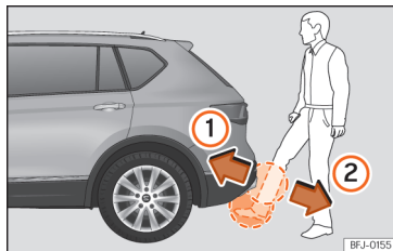
Fig. 79 Rear lid with sensor-controlled opening (Easy Open).
