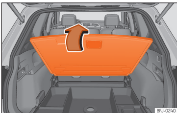
Fig. 199 In the boot: lift the boot floor.
