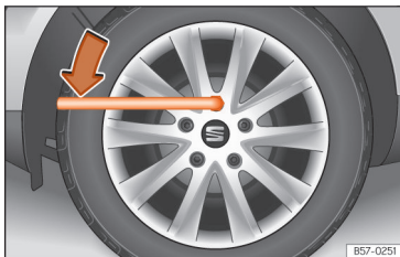
Fig. 253 Tyre change: slacken the wheel bolts.
