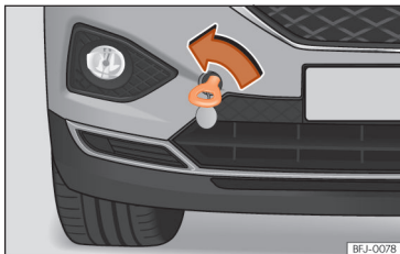
Fig. 226 Right side of the front bumper: towline anchorage screwed in.
