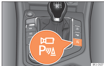
Fig. 171 Centre console: button to manually switch on/off the Top View camera system when in combination with the parking assist system.
