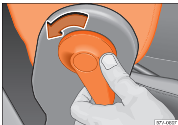
Fig. 91 Unlocking the folding backrest of the front passenger seat
