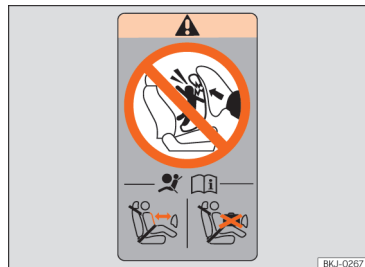
Fig. 41 Airbag sticker: on the rear frame of the passenger side door.
