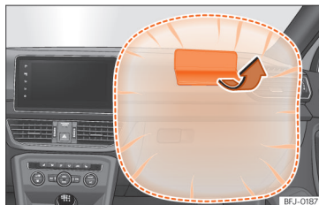
Fig. 32 Front passenger airbag located in dash panel.
