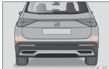
Fig. 135 Rear view of the vehicle: radar sensor areas.
