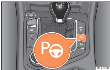
Fig. 162 In the centre console: button to switch on the Park Assist system.
