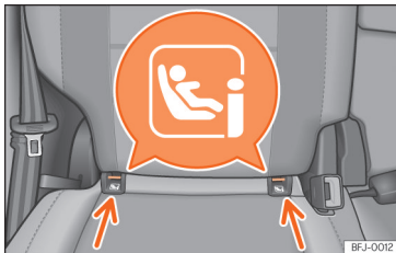
Fig. 42 Rear seat: location of the ISOFIX or i-Size securing rings.
