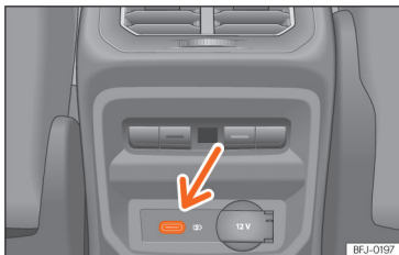
Fig. 186 Rear centre console: USB connectors with power socket function.
