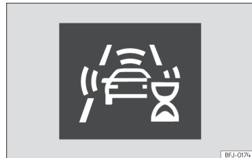
Fig. 146 On the instrument cluster screen: indication of the system's initial self-calibration.
