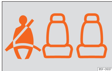
Fig. 22 Instrument cluster: indication of the status of the rear seat seat belts.
