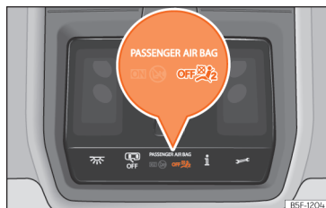
Fig. 32 On the roof console: passenger airbag deactivation control lamp.
