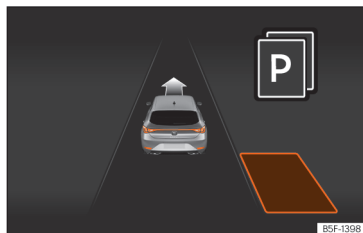
Fig. 157 On the instrument panel display: display of the assisted parking system with decreased visibility.
