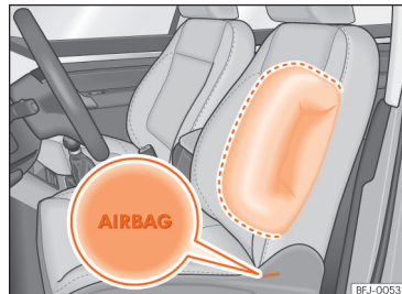
Fig. 35 Side airbag in driver's seat.
