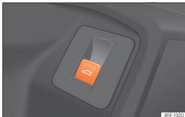
Fig. 82 On the driver's door: button for opening and closing the rear lid.
