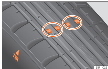
Fig. 239 Tyre profile: tread wear indicators.
