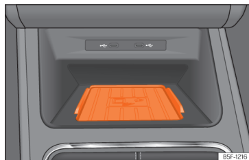
Fig. 179 On the centre console: pad for the mobile phone connection.
