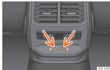
Fig. 172 Rear centre console: USB connectors with power socket function.
