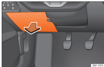
Fig. 221 On the dashboard on the driver side: lid of the fuse box.
