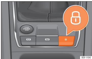
Fig. 76 On the centre console: central locking button
