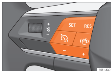
Fig. 132 On the multifunction steering wheel: cruise control operation buttons.
