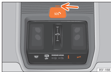
Fig. 52 On the roof console: controls for voice services.
