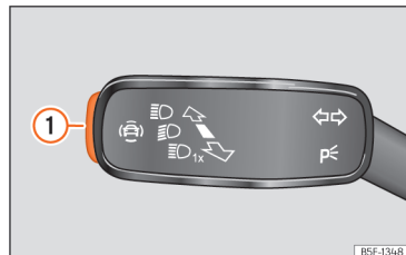
Fig. 124 On the turn light and main beam lever: key for driver assistance systems [depending on the version].
