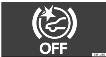
Fig. 144 On the screen of the instrument panel Front Assist switched off message.
