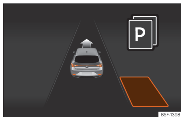
Fig. 151 On the instrument panel display: display of the assisted parking system with decreased visibility.
