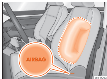
Fig. 36 Side airbag in driver's seat.
