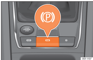
Fig. 147 Centre console, lower part: electronic parking brake button.
