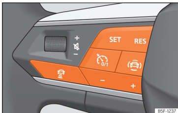
Fig. 132 On the multifunction steering wheel: buttons for operating the ACC.
