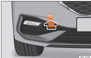
Fig. 211 Front bumper on right: remove the lid.
