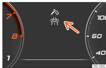
Fig. 13 Eco-efficient driving assistance indication (schematic representation).
