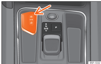
Fig. 67 Centre console: vehicle key housing.
