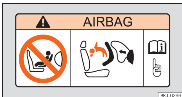
Fig. 42 Airbag sticker: on the passenger side sunshade blind.
