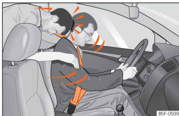
Fig. 25 Any rear seat occupants not wearing a seat belt may be thrown forward violently, hitting the driver who is wearing the seat belt.
