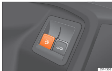
Fig. 203 Driver's door: tank cover release.
