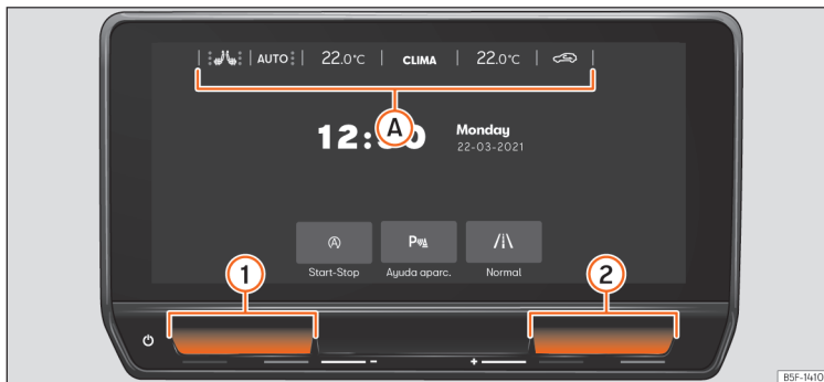
Fig. 111 Schematic representation: air-conditioning functions.
