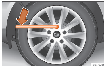
Fig. 240 Tyre change: slacken the wheel bolts.
