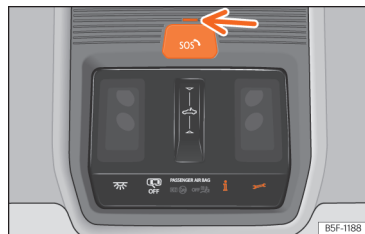
Fig. 53 On the roof console: controls for voice services.
