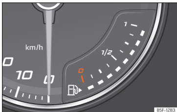
Fig. 6 Analogue instrument cluster: fuel gauge
