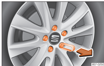
Fig. 238 Wheel: wheel bolts with caps.
