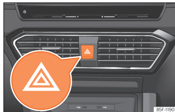
Fig. 52 Dashboard: switch for hazard warning lights.
