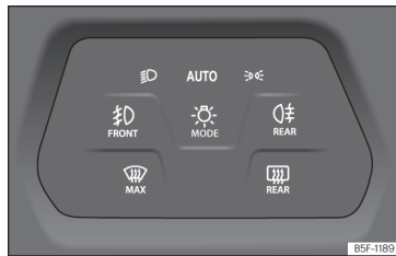
Fig. 101 Instrument panel: light panel.
