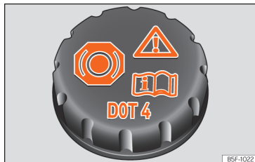
Fig. 223 Engine compartment: brake fluid reservoir cap.
