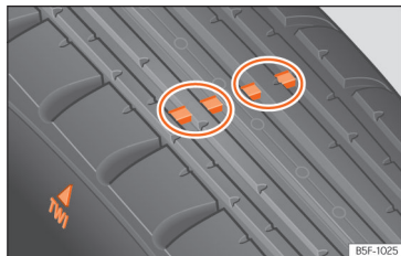
Fig. 233 Tyre profile: tread wear indicators.
