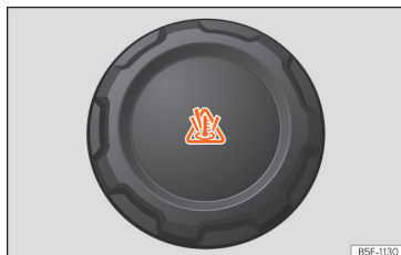
Fig. 222 Front compartment: coolant expansion tank cap.
