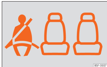
Fig. 20 Instrument cluster: indication of the status of the rear seat seat belts.
