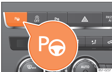
Fig. 138 In the centre console, top section: button to switch on the Park Assist system.
